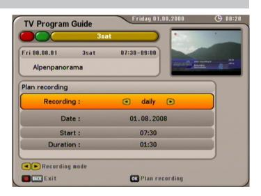
When all settings have been made, press the button to save the recording settings. You can view the scheduled recording in the timer list view of the EPG (see section "Timer list").
